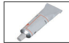
Electrical Grade Silicone Glue Required to attach accessories to Border Tube properly. Improper coverage or unapproved silicone will void warranty. 8 minutes tack-free time; silicone glue will take 24-72 hours to cure. Keep uncured silicone away from open flame.
